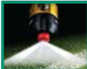
The Deluxe version features a solenoid triggered spray head. This enhances the atomisation of the paint compared to the standard diaphragm controlled spray head. This improves leaf coverage, without any increase in paint usage, and gives instant shut-off of paint to the spray head. This eliminates over-spray at the end of the marked line.
